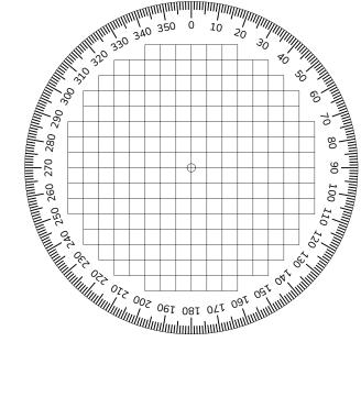
Print me on overhead transparancy. Cut out the protractor and base plate. Use a pin to create a hole in the centre of each (using the guide).
